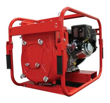
The self primping pump "Trash" is designed to comply to the hardest and heavy duty applications expecially for emergency when there is dirty sewage and muddy water with the presence of solids and sand. The open-blade impeller ensures a superior priming ability voiding the need of a foot valve installation. The high thickness of the pump body and of the impeller blades, allow the handling of more abrasive fluids and large passage of solids.
